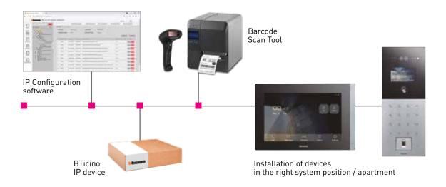
The label on the devices allows to associate them in the topology using a scan tool in a very easy and quick way. The system will then print a label, with all the position information, to be attached to the packaging. This will guarantee error-proof installation.
